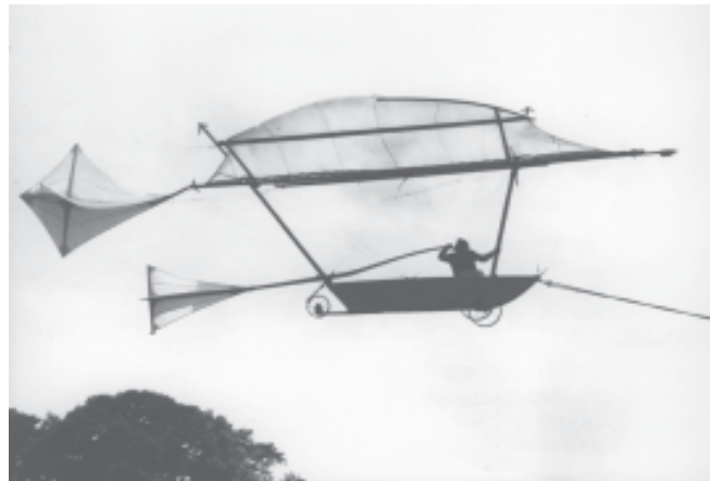
Fig 2-2 Reproduction of the Cayley glider (photo courtesy of RAF Museum).
